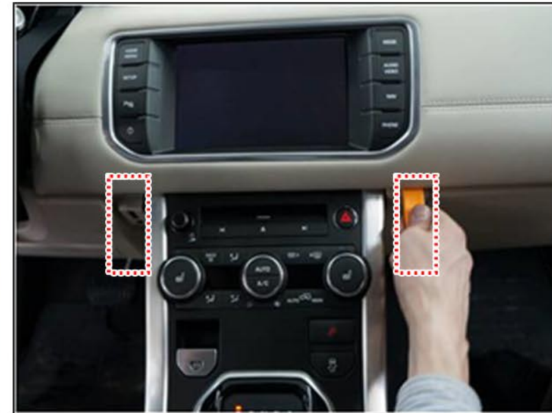
Open those covers and remove bolts holding them.
