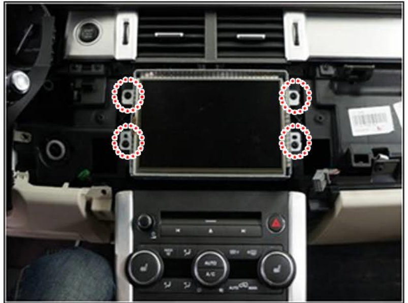
Remove those 4 bolts holding Monitor Display.
