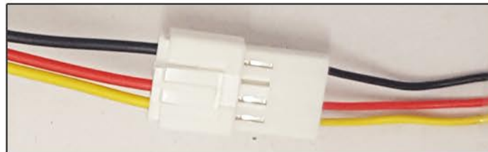
4 Pin Joint Connection
